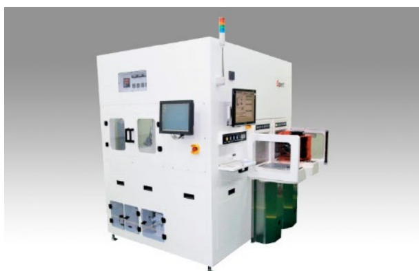
IAS's main product, Expert (Fully automated equipment for testing by VPD)
