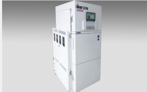
CO<sub>2</sub> Incubator with medium exchange
