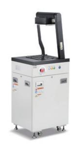
ALP is placed next to 300 mm load ports, can receive FOUPs from OHTs and pass them to load ports.
